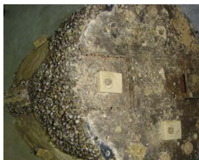
A 3 year old SeaBat 7101 which has not been maintained regularly
